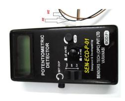
SEN-ECD-P-01 is equipped with inbuilt two electrode connector specially designed for precise connecting to potentiometric electrochemical cell. In addition system may be usable with all kind
